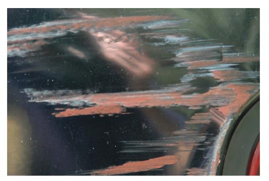
Another bit of evidence that can be helpful in determining the orientation of the vehicles or even which vehicle hit another vehicle at different points in a multi-vehicle accident is paint transfer. Many times paint from one vehicle will be transferred onto the other vehicle where they make contact. Although many times this evidence may be obvious there are other times where it is very miniscule and requires careful examination.
