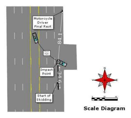
The takeoff angle for a motorcycle operator is generally between 10 to 20 degrees. The takeoff angle for the passenger varies depending on the type of motorcycle and operator position of the particular accident and can be as low as 18 to 20 degrees and as much as 45 degrees.
