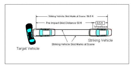
The striking vehicle left 59.5 feet of pre-impact skid marks and had a wheel base distance of 9.5 feet. Subtracting the wheelbase distance from the total skid mark distance gives a pre-impact skid distance of 50 feet. The skidding occurred on a roadway that was level, dry asphalt. The drag factor was measured to be .7 g's. The vehicle impacted into the side of another car and left 18 inches (1.5 feet) of permanent crush damage.
